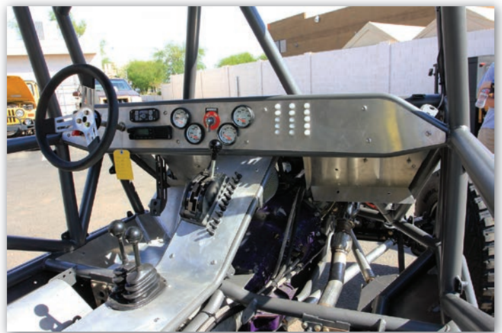
LetzRoll fabricated this vehicle with 2" diameter, .120" wall chrome-moly tubing. It ran in the 4800 class at King of the Hammers.
